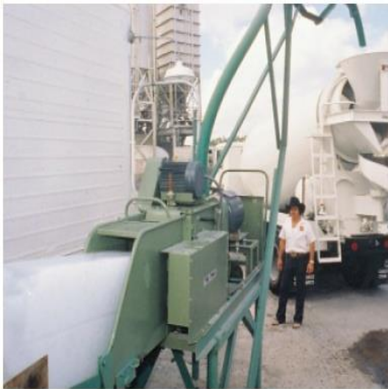
Fig. 13-6. Substituting ice for part of the mixing water will substantially lower concrete temperature. A crusher delivers finely crushed ice to a truck mixer reliably and quickly. (IMG12265)
