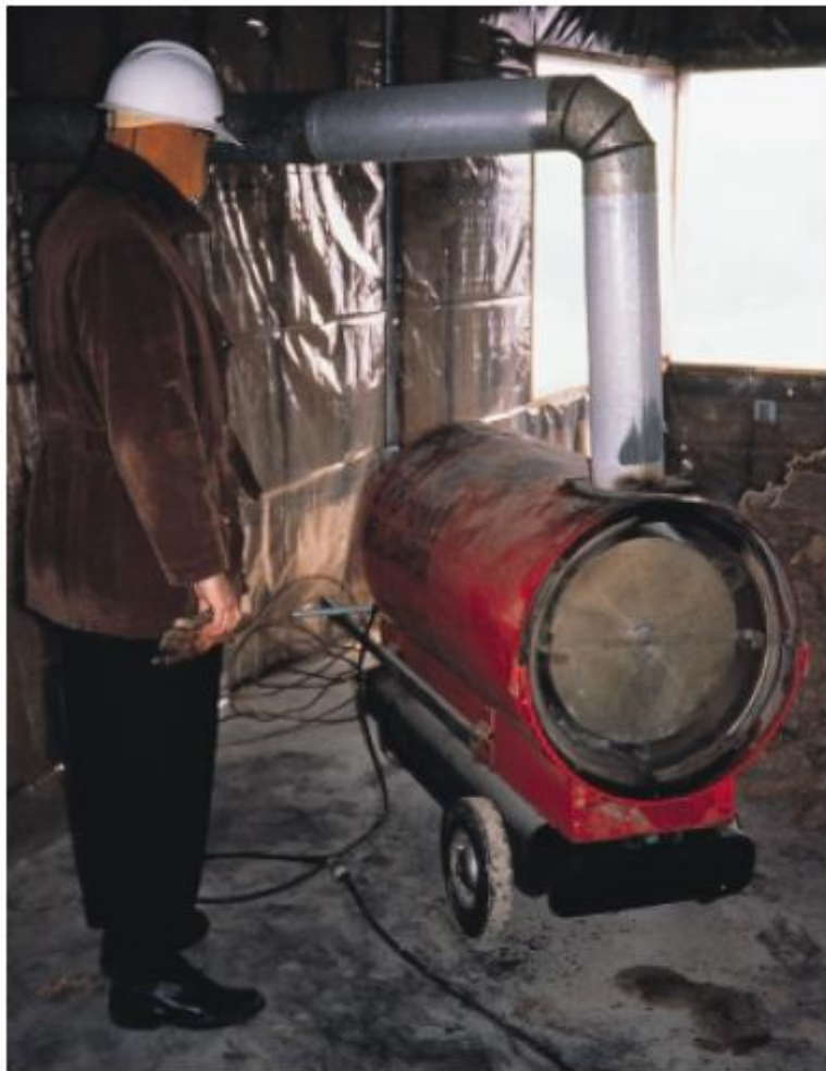
Fig. 14-23. An indirect-fired heater. Notice vent pipe that carries combustion gases outside the enclosure. (IMG12275)
