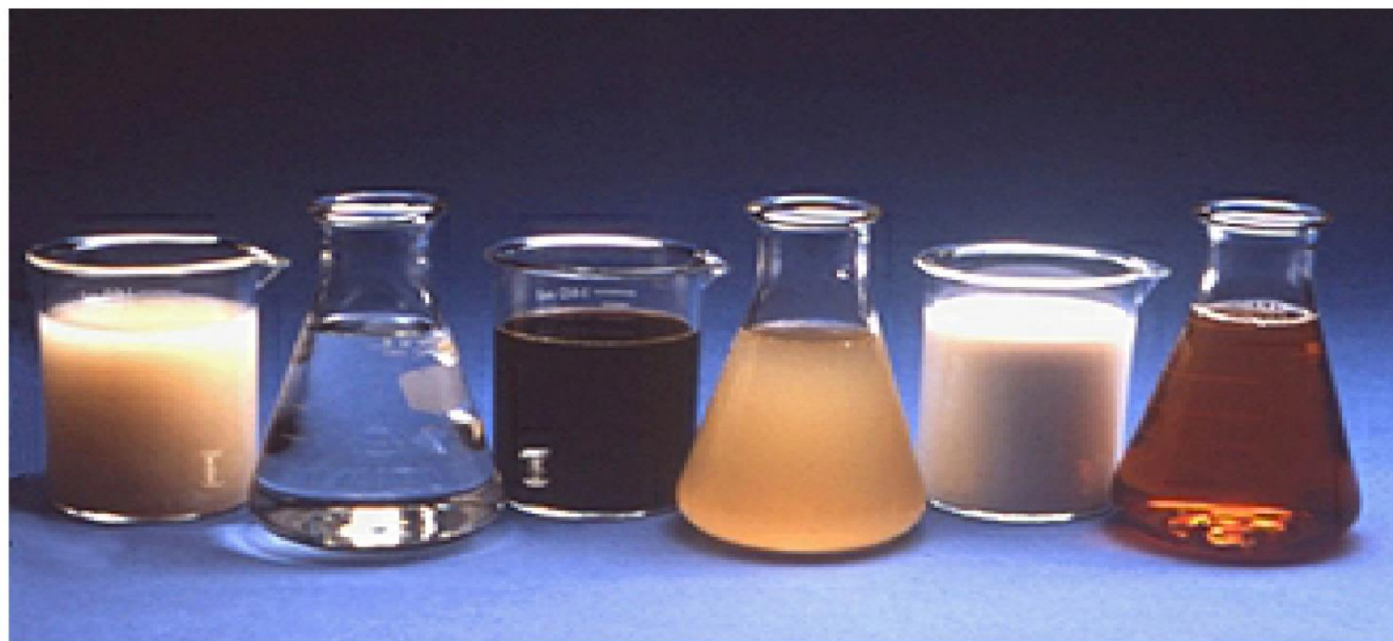
Fig. 6-1. Liquid admixtures, from left to right: antiwashout admixture, shrinkage reducer, water reducer, foaming agent, corrosion inhibitor, and air-entraining admixture. (IMG12188)
